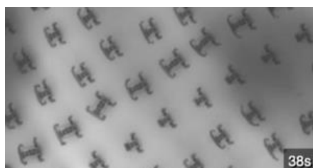
Figure 48. Four-Legged Reduced Graphene Oxide or Graphene Hydroxide Nanobots. 140 The micro-robots shown above feature four legs and are composed of hexagonal reduced graphene oxide or graphene hydroxide which are highly magnetic, flexible and super strong. This enables the Reduced Graphene Oxide or Graphene Hydroxide nanobots to carry a body which weighs about 8000 times more than each leg. As well, each leg measures only 100 atoms and even down to 1 atom thick, and they can carry bodies 1000 to 100000 times thicker. 141
